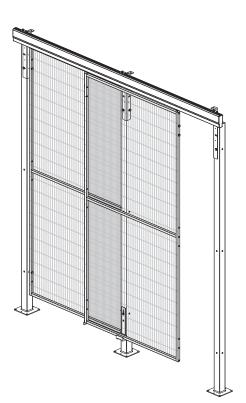
Sliding door suspended by means of a new generation upper guide. Ergonomic and functional, it is simple to assemble and ensures a smooth opening movement.
